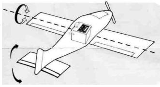
•When the gyro is mounted 180° out of phase, the direction of the correcting mix will be reversed. To correct this situation, switch the internal reverse amp switch to "REV". After mounting the gyro to the fuselage, recheck its direction of operation.
